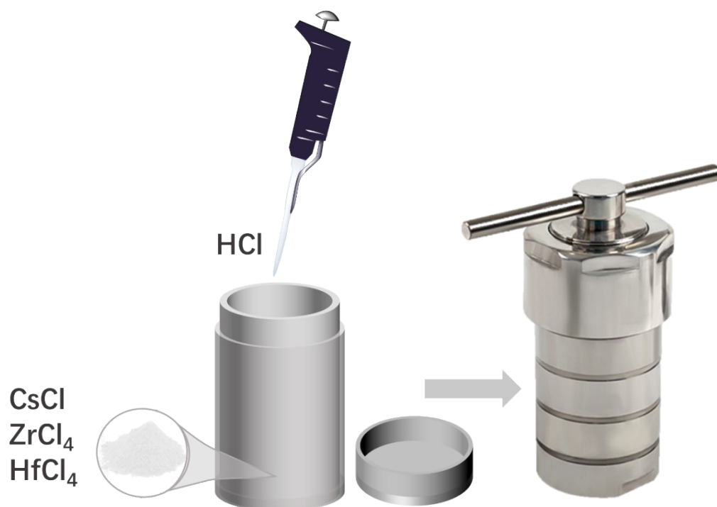
Figure S1. Schematic diagram of the synthesis process of Cs 2 ZrCl 6 ·xHf powders by solvothermal method.
