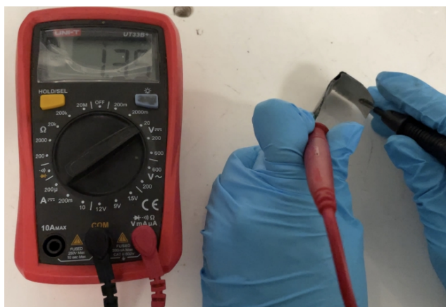
Fig. S20. Photograph of the open-circuit voltage of a flexible solid-state ZAB assembled with FeNi/NC@Ti 4 O 7 -CNFs as air cathodes under bending conditions.
