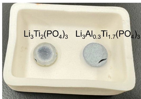
Figure S1 – Appearance of \text{Li}_3\text{Al}_x\text{Ti}_{2-x}(\text{PO}_4)_3 ( x=0, 0.3 ) (a) Before heating; (b) after heating at 925 °C under Ar for 2 h with heating and cooling rates of 5 °C \text{min}^{-1} .
