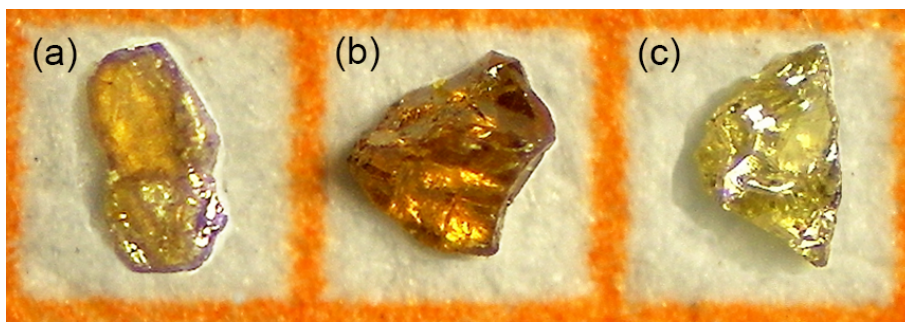
Figure S1. Morphologies of \text{Ag}_2\text{CdSiS}_4 (a), \text{BaAg}_2\text{SiS}_4 (b) and \text{LaAgSiS}_4 (c) crystals in 1\text{mm}^2 reference dimension.
