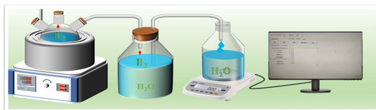
Fig. S9. Schematic diagram of the setup for \text{H}_2 production by hydrolysis of 150 mM \text{NaBH}_4 + 0.4 wt.% \text{NaOH} solution.
