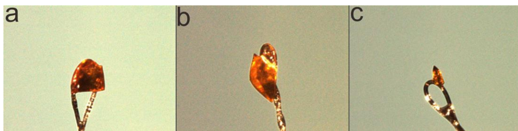
Fig. S17 Photographs of single crystals of \text{Pd}_4\text{S}_2 . (a) Achiral space group P_{21/n} ; (b) Chiral space group with Flack parameter of 0.5; (c) Chiral space group with Flack parameter of zero.
