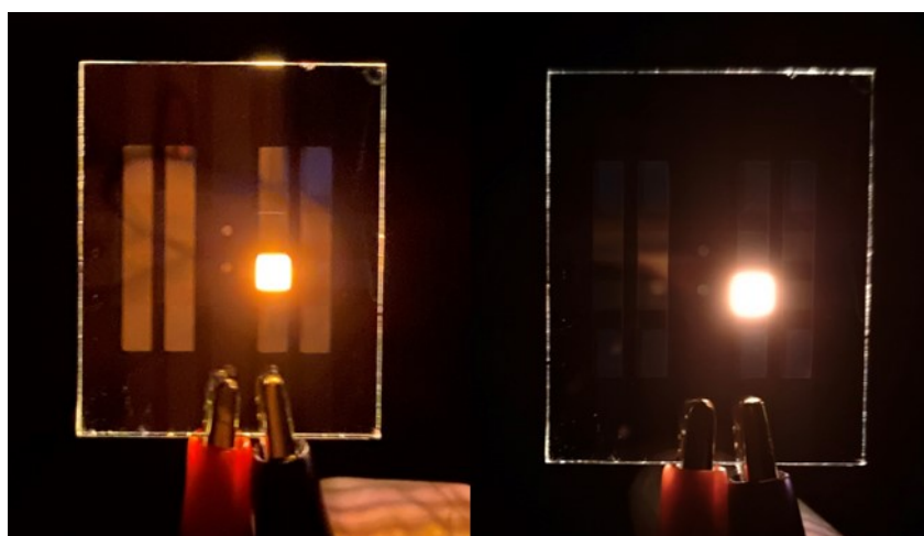
Figure S40. OLED devices using complex 1 .
