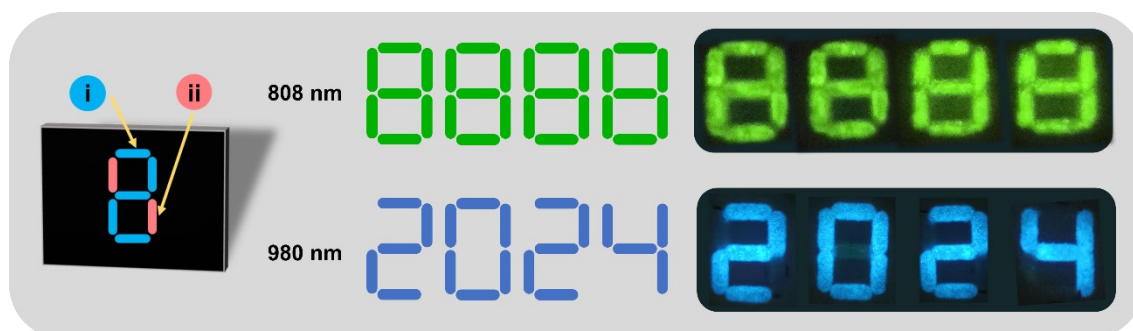
Figure S12. Demonstration the double-color emissions of the construction of four 8-shaped pattern using \text{NaErF}_4@\text{NaYF}_4:\text{Eu}^{3+} nanoparticles and \text{NaErF}_4@\text{NaYF}_4:\text{Eu}^{3+}@\text{NaBiF}_4:\text{Yb}^{3+},\text{Tm}^{3+} nanoparticles. (i): \text{NaErF}_4@\text{NaYF}_4:10\% \text{Eu}^{3+} and \text{NaErF}_4@\text{NaYF}_4:10\% \text{Eu}^{3+}@\text{NaBiF}_4:\text{Yb}^{3+},\text{Tm}^{3+} nanoparticles. (ii): \text{NaErF}_4@\text{NaYF}_4:10\% \text{Eu}^{3+} nanoparticles.
