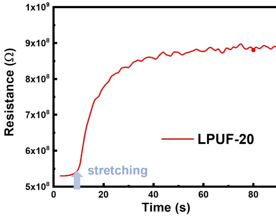
Figure S3. LPUF-20 resistance curve during the test.
