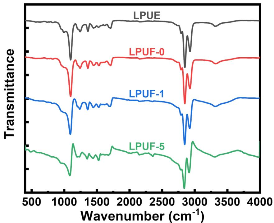
Figure S2. FTIR spectra of the LPUE and LPUF.
