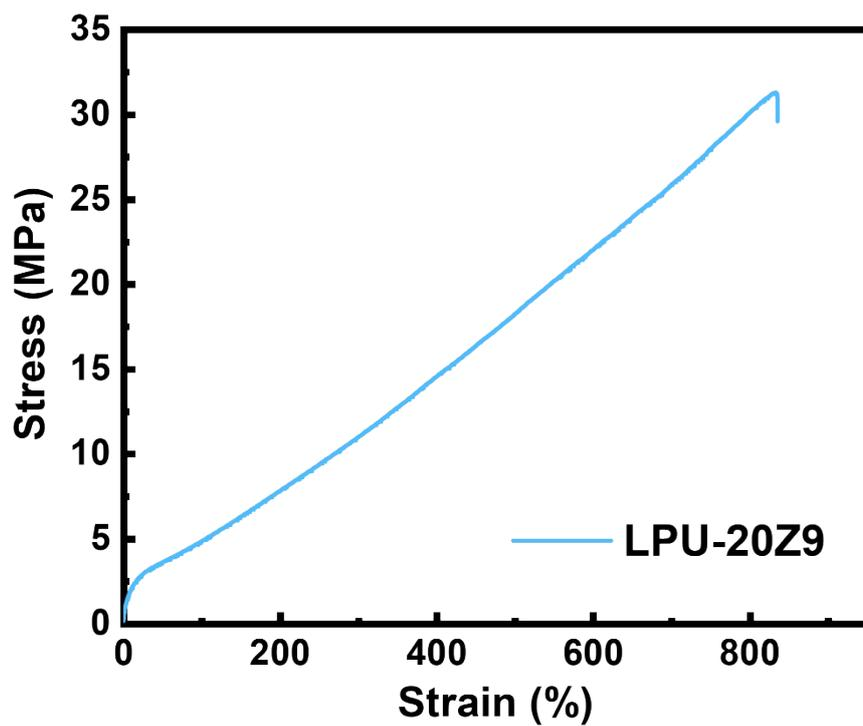
Figure S1. Representative stress-strain curves of LPUE.
