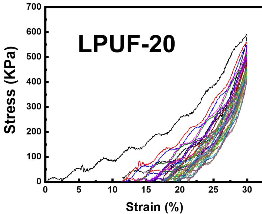
Figure S4. Cyclic stress-strain curve of LPUF-20
