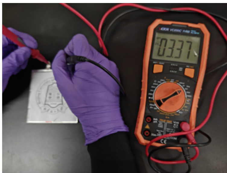
Fig. S14 Open circuit voltage of a pouch cell.
