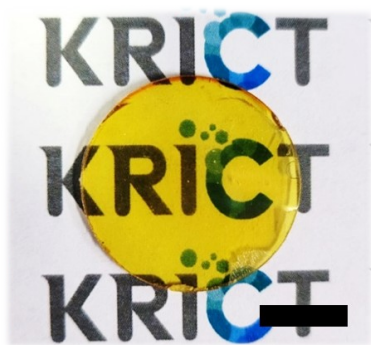
Fig. S15. Digital image of window made from S80T20 thermally treated for 12 h at 140 °C. (Dia. 25 mm × thickness 1 mm). Scale bar for the image is 1 cm.
