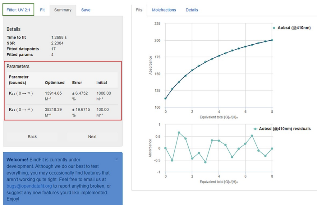
Fig. S4. Screenshot of the summary window of http://app.supramolecular.org/bindfit/ . This screenshot shows the raw data for fluorescence titration of Py-CT4 with \text{HSO}_4^- following the fluorescence emission values at 410 nm vs. the data fitted to a 2:1 UV binding model, the corresponding residual plot and the association constants with the calculated asymptotic standard errors.
