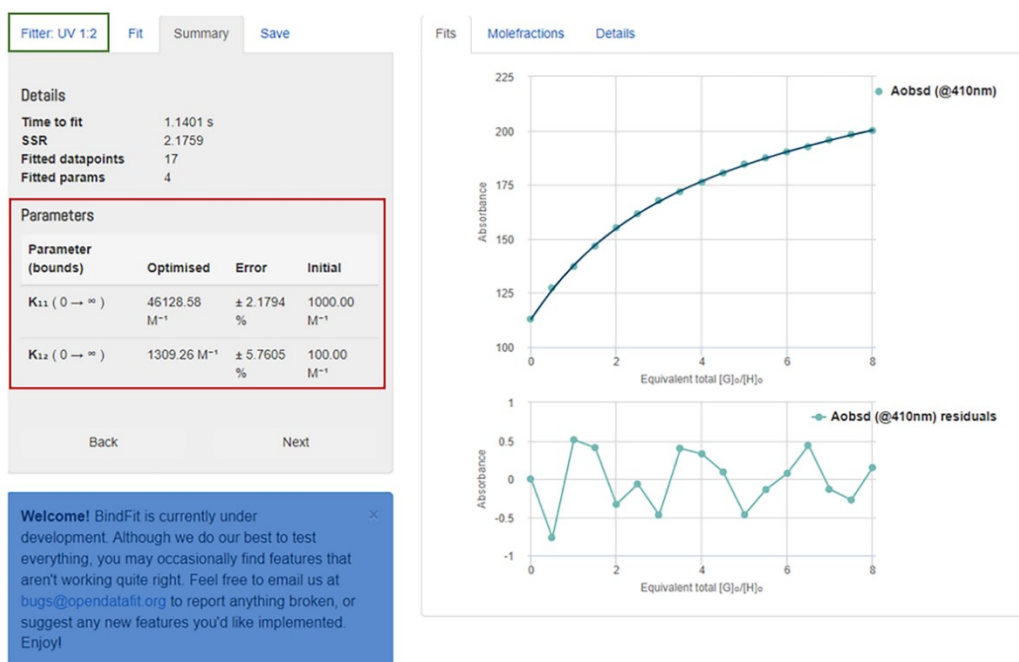
Fig. S3. Screenshot of the summary window of http://app.supramolecular.org/bindfit/ . This screenshot shows the raw data for fluorescence titration of Py-CT4 with \text{HSO}_4^- following the fluorescence emission values at 410 nm vs. the data fitted to a 1:2 UV binding model, the corresponding residual plot and the association constants with the calculated asymptotic standard errors.
