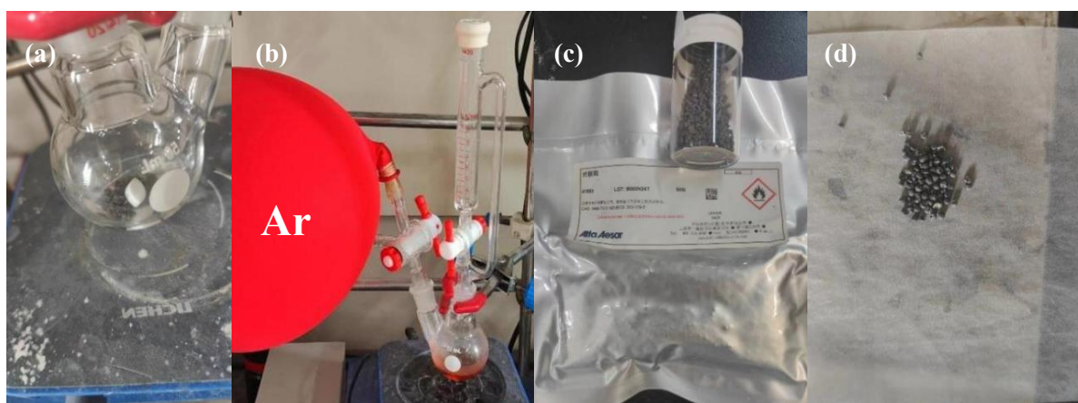
Figure S3 Reaction set-up for Ca-promoted reductive silylation. (a) Before calcium activation; (b) General reaction setup; (c) Commercially available calcium granules; (d) Calcium granules size \sim 2 mm.
