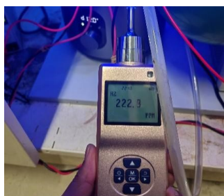
Figure S3. H 2 detection experiment by a H 2 detector for the synthesis of 6a after 3 hours.
