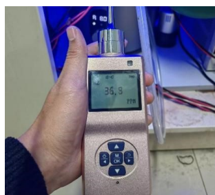
Figure S2. H 2 detection experiment by a H 2 detector for the synthesis of 3a after 3 hours.
