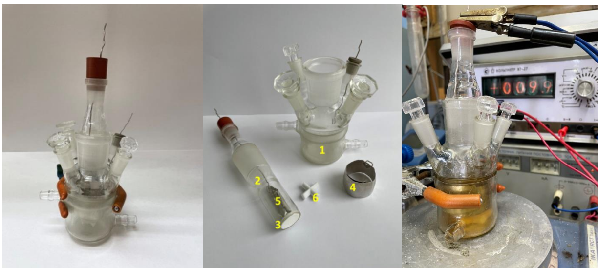
Figure S1. Electrolysis setup: cylindrical cell with divided anodic and cathodic compartments. 1 - anodic compartment; 2 - cathodic compartment; 3 - membrane: ceramic plate with the pore size of 900 nm; 4 – platinum cylindrical working electrode with a surface area of 20 cm 2 (anode); 5 - platinum rod (10 cm 2 ) (cathode); 6 - stir bar. The cell can be thermostatted.
