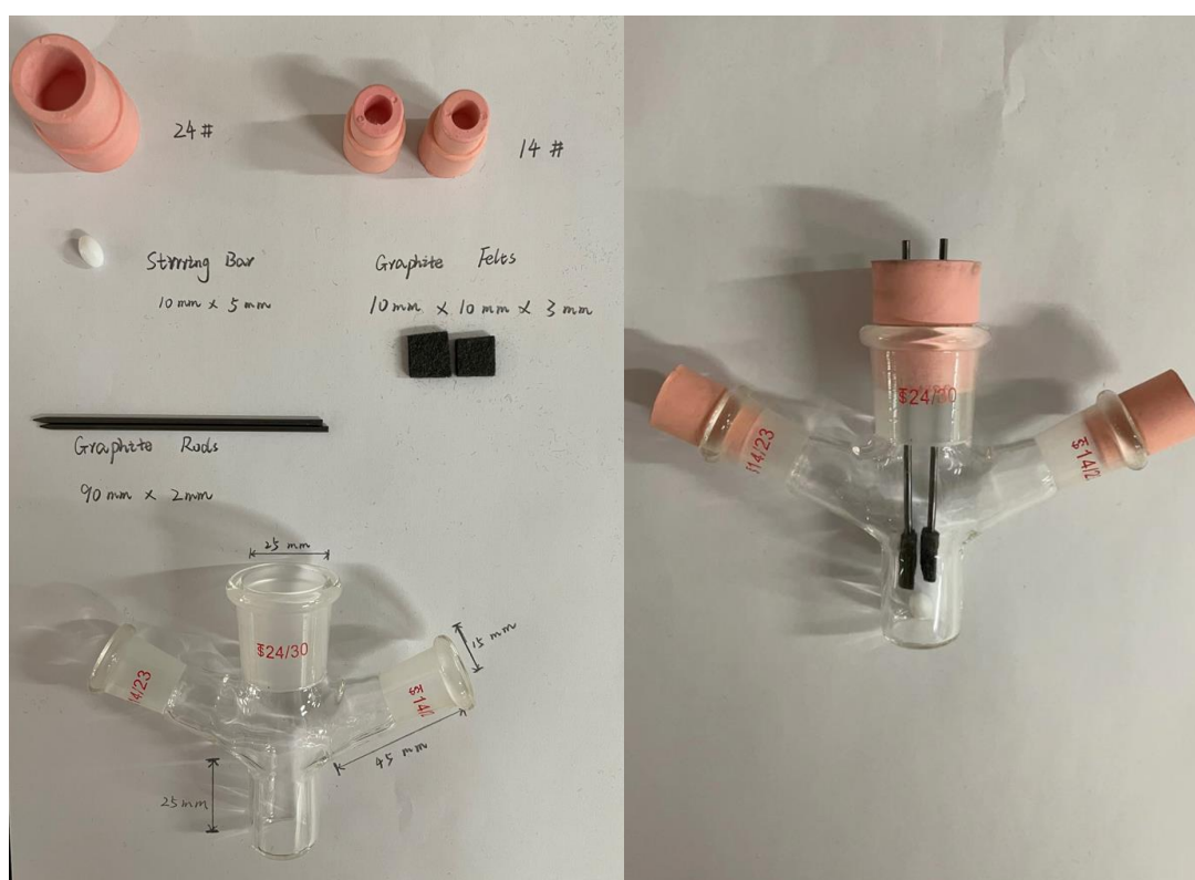
Figure S1. List and Assembly of Electrochemical Experimental Materials
