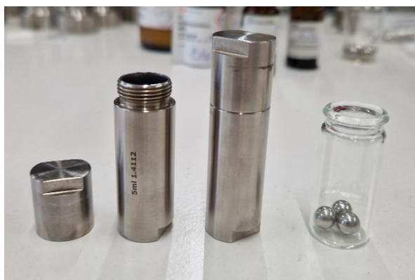
Figure S2. 5 mL jars and 7 mm balls
