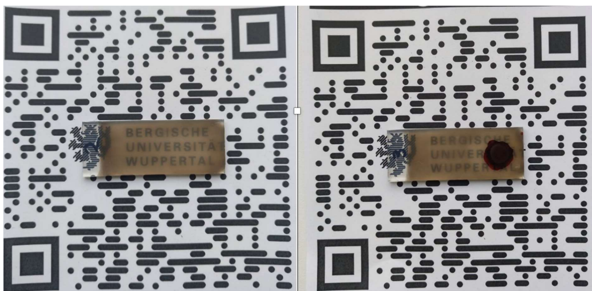
Figure S 49: Nickeloxide-nanoflakes on the FTO-substrate before (left) and after dropcasting the Copolymers on a 0.785 cm 2 large area (right).
