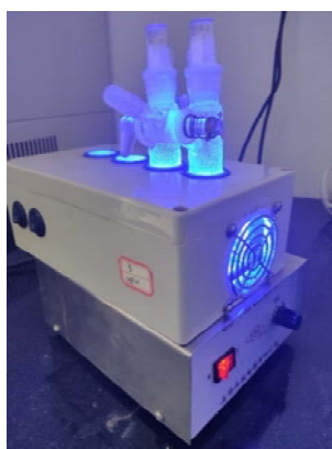
Figure S1. Setup of the photochemical reaction.
