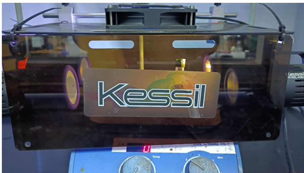
Figure S2. Dedicated Kessil photo reactor used in this work
