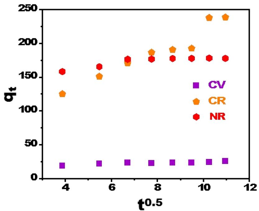
**Figure S6.** Modeling of uptake kinetics for CV, CR, and NR dyes with simplified model of resistance to intraparticle diffusion (Morris and Weber equation).
