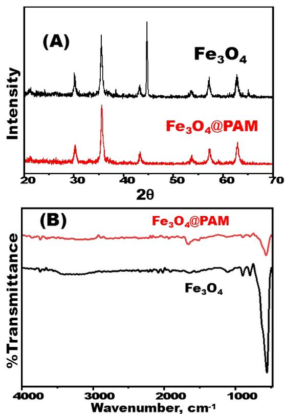
**Figure S1.** The magnetite  $\text{Fe}_3\text{O}_4$  and  $\text{Fe}_3\text{O}_4$ @PAM (A) PXRD diffraction patterns . B) FTIR spectra of magnetite  $\text{Fe}_3\text{O}_4$  and  $\text{Fe}_3\text{O}_4$ @PAM.
