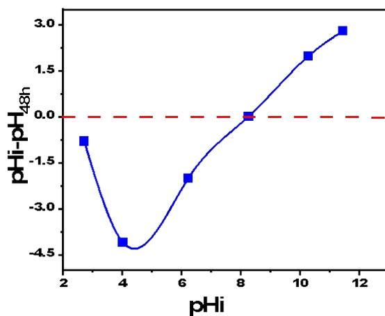
**Figure S4.** Variations in pH for to identify the isoelectric point of MDLZ magnetic nanocubes adsorbent.
