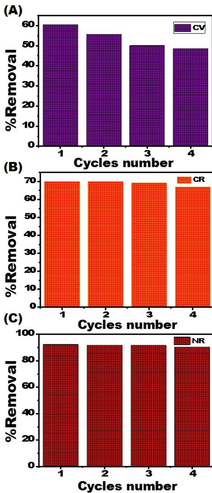
**Figure S7.** The adsorption, elution and regeneration of nanocubes MDLZ adsorbent for multiple cycles of A) CV, B) CR, and C) NR dyes.
