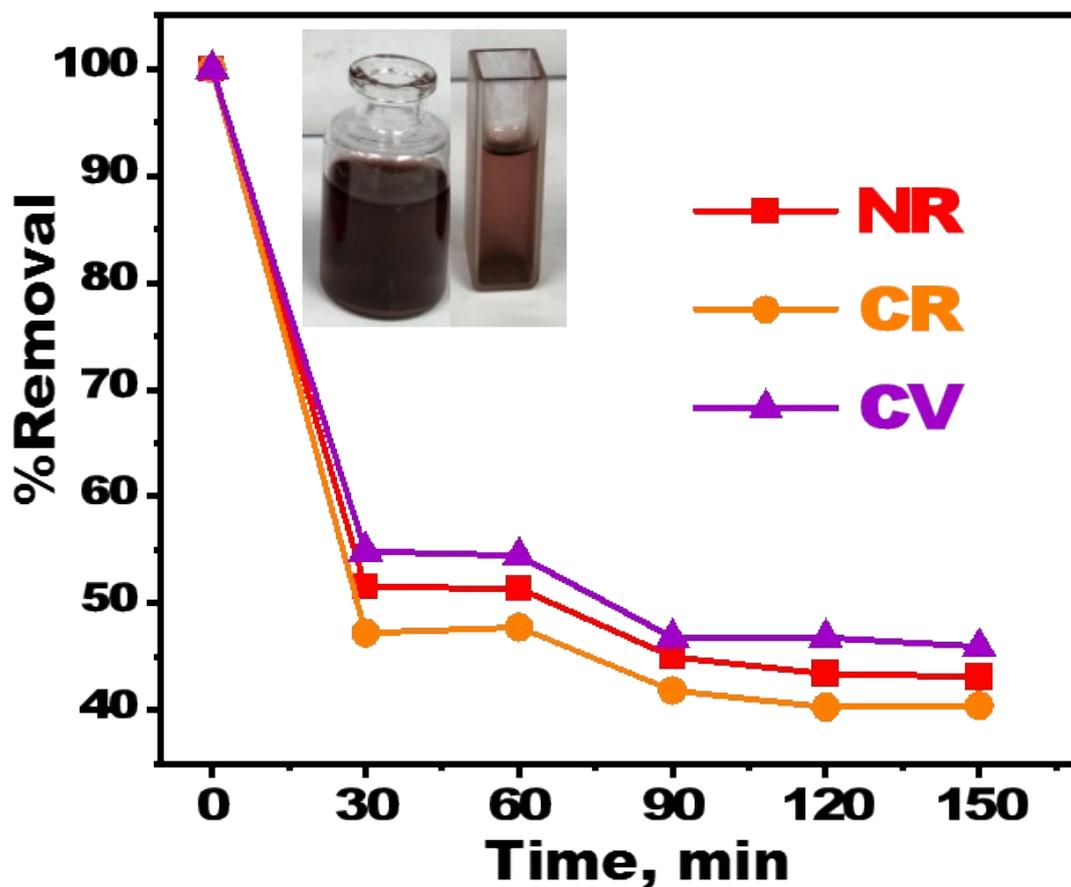
**Figure S8.** The adsorption of multiple dyes using nanocubes MDLZ adsorbent in simulated solution containing different concentration of cationic and anionic dyes.
