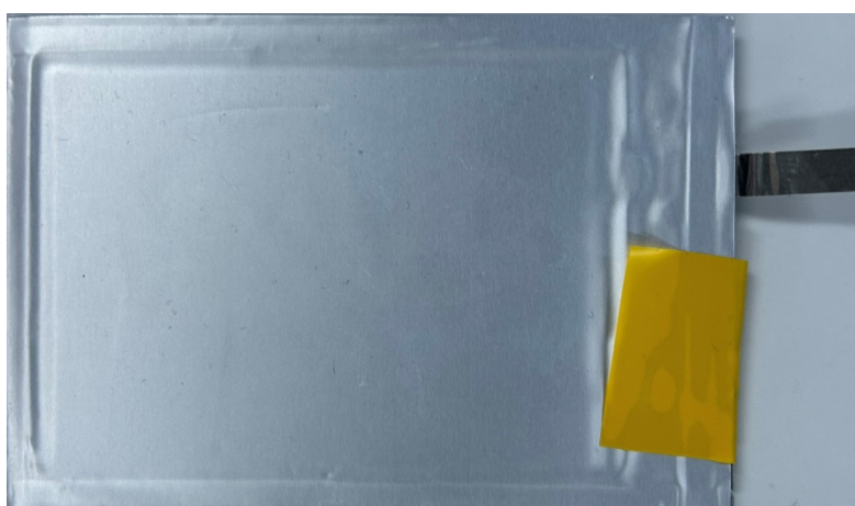
Fig.1 The photo of the pouch cell for cycling tests.
