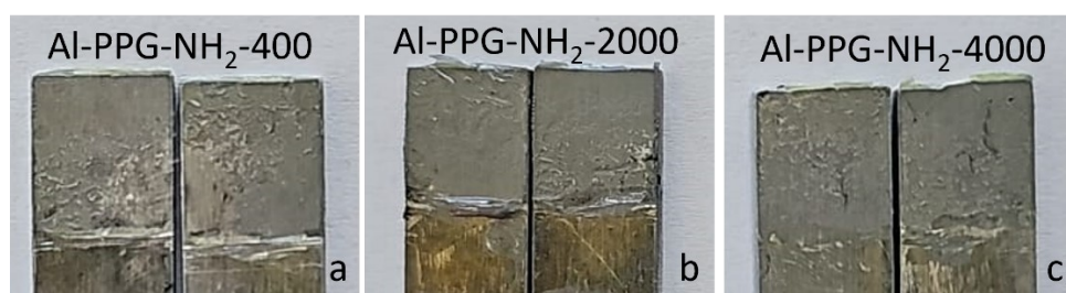
Figure S3. The post-fracture macro-images of the Al-PPG-NH 2 -400 (a), Al-PPG-NH 2 -2000 (b), and Al-PPG-NH 2 -4000 (c) specimens
