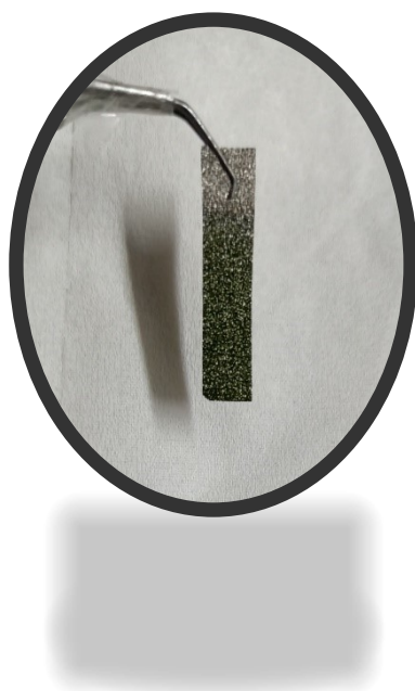
Fig. S1: Digital picture of electrodeposited PANI electrode.
