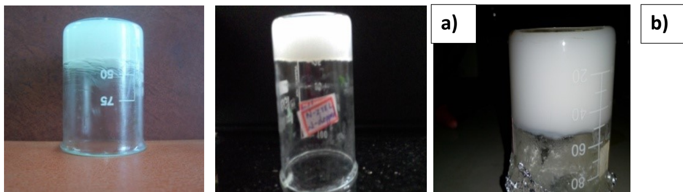
Fig. S6 Photographic images a) C-ZnO b) N-ZnO & c) S-ZnO gel sample.
