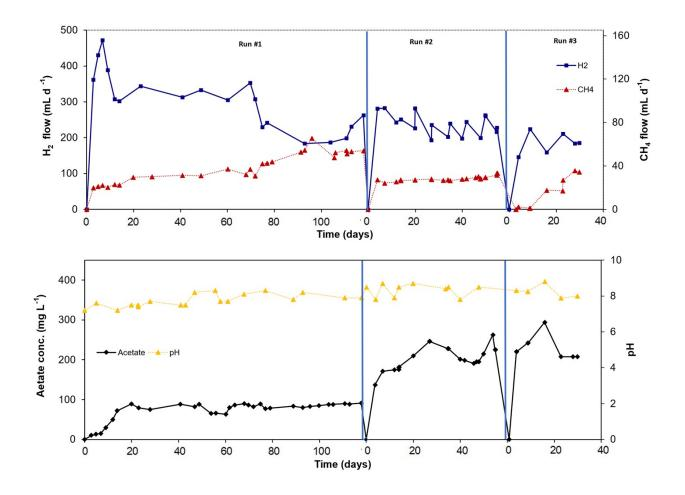
Figure S3: Time dependence of (A)  $CH_4$  and  $H_2$  production rate, (B) Acetate concentration and pH in the cathode compartment of MES-2 cell.
