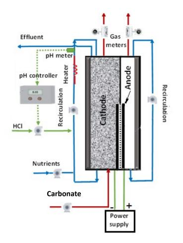
**Figure S1.** Schematic representation of a MES cell with continuous carbonate supply. The dotted line denotes PEM. Figure adapted from Gomez Vidales et al<sup>37</sup>.
