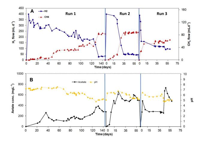
**Figure S2**: Time dependence of (A)  $CH_4$  and  $H_2$  production rate, (B) Acetate concentration and pH in the cathode compartment of MES-1 cell.
