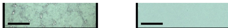
S6 Microscopic images of parts of the HCCMs fabricated using the inks with roller mixer parameter variation. Images taken with a confocal microscope from WiTeC using a 5x, Zeiss EC “Epiplan” objective. Black bars represent a scale of 500 \mu\text{m} . The images depict the agglomeration scale within the catalyst layers as well as the number and size of pores.
