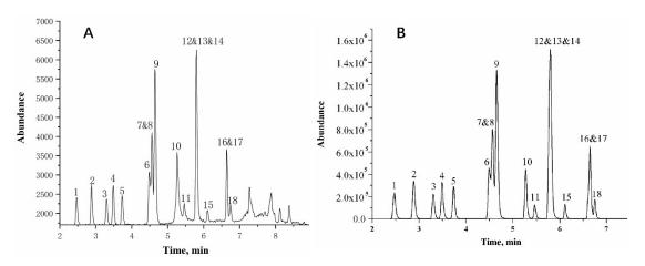
Fig.2. The total ion flow chromatogram of LOD (  $0.1\mu g/kg$ , A ) and a standard solution with a concentration of 20  $\mu g/L$  (B).
