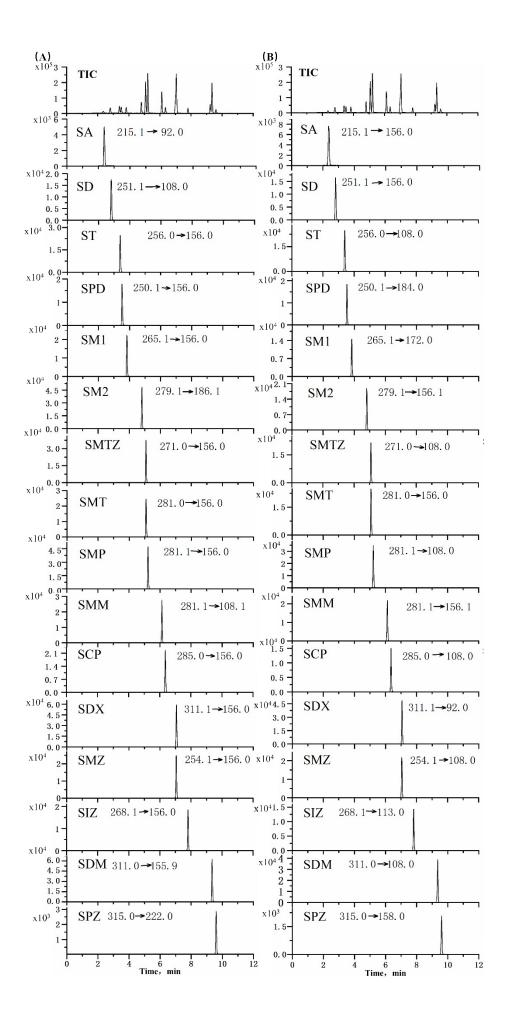
Fig.1. The selective ion chromatograms for each sulfonamide of blank forage grasses matrix spiked at 20  $\mu$ g/L. The A represents a quantitative ion pair chromatogram, while B denotes a qualitative ion pair chromatogram.
