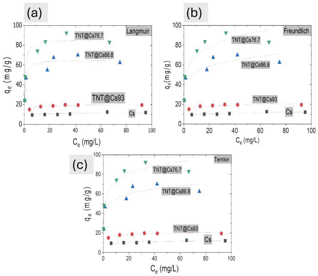
**Figure S2:** The non-linear isotherm curves for the (a) Langmuir, (b) Freundlich, and (c) Temkin models.
