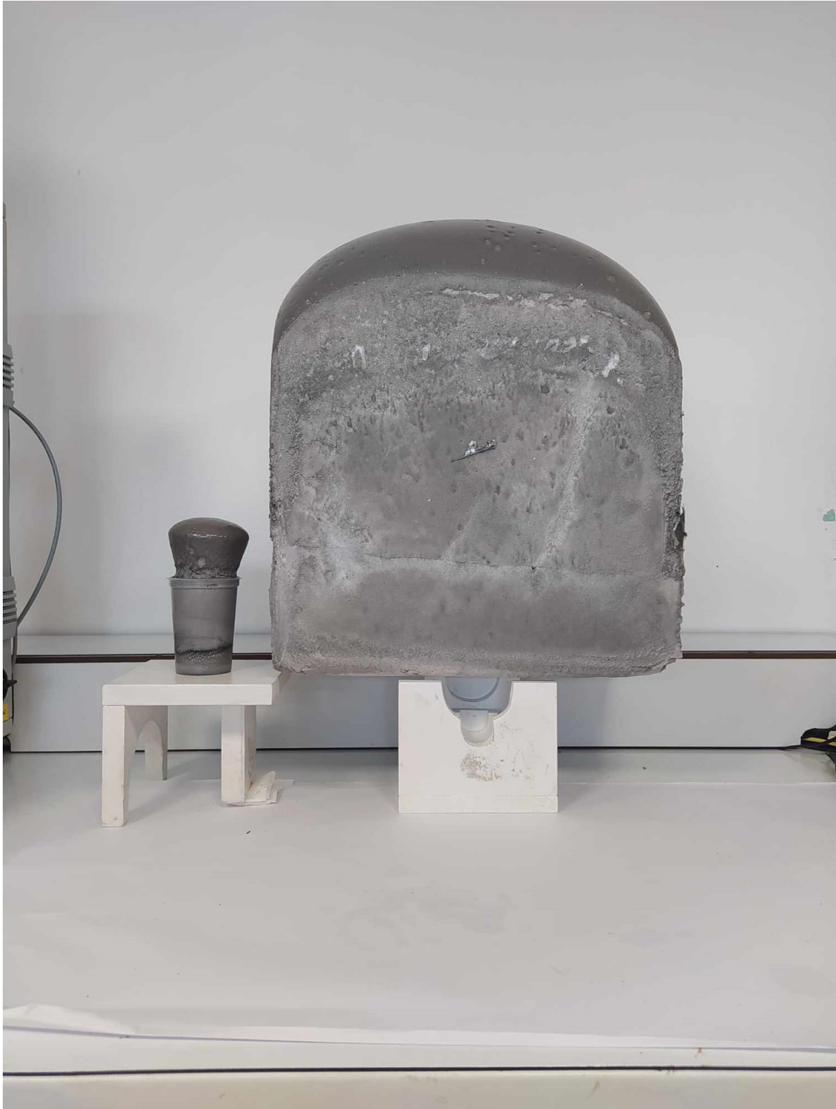
Figure S16. The quantity comparison of 565 ml cup PUR and 125 L PUR mini block containing 20 wt.% of the PUR liquid recycle.
