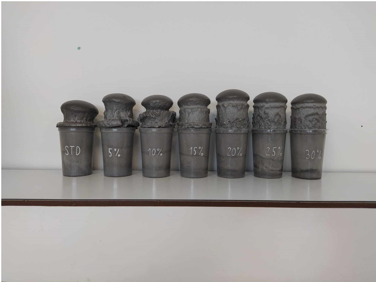
Figure S15. The formed PUR cups from the performed cup tests. The percentage on the cup marks the wt.% amount of the PUR liquid recyclate in the foam.
