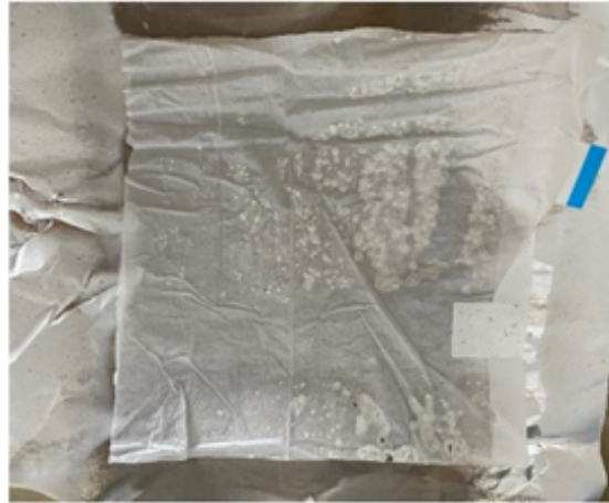
Supplementary data file 07: (a) The process of the electrospinning on the surface of a diaper and (b) Resulted nanofiber mat on the surface of the diaper.
