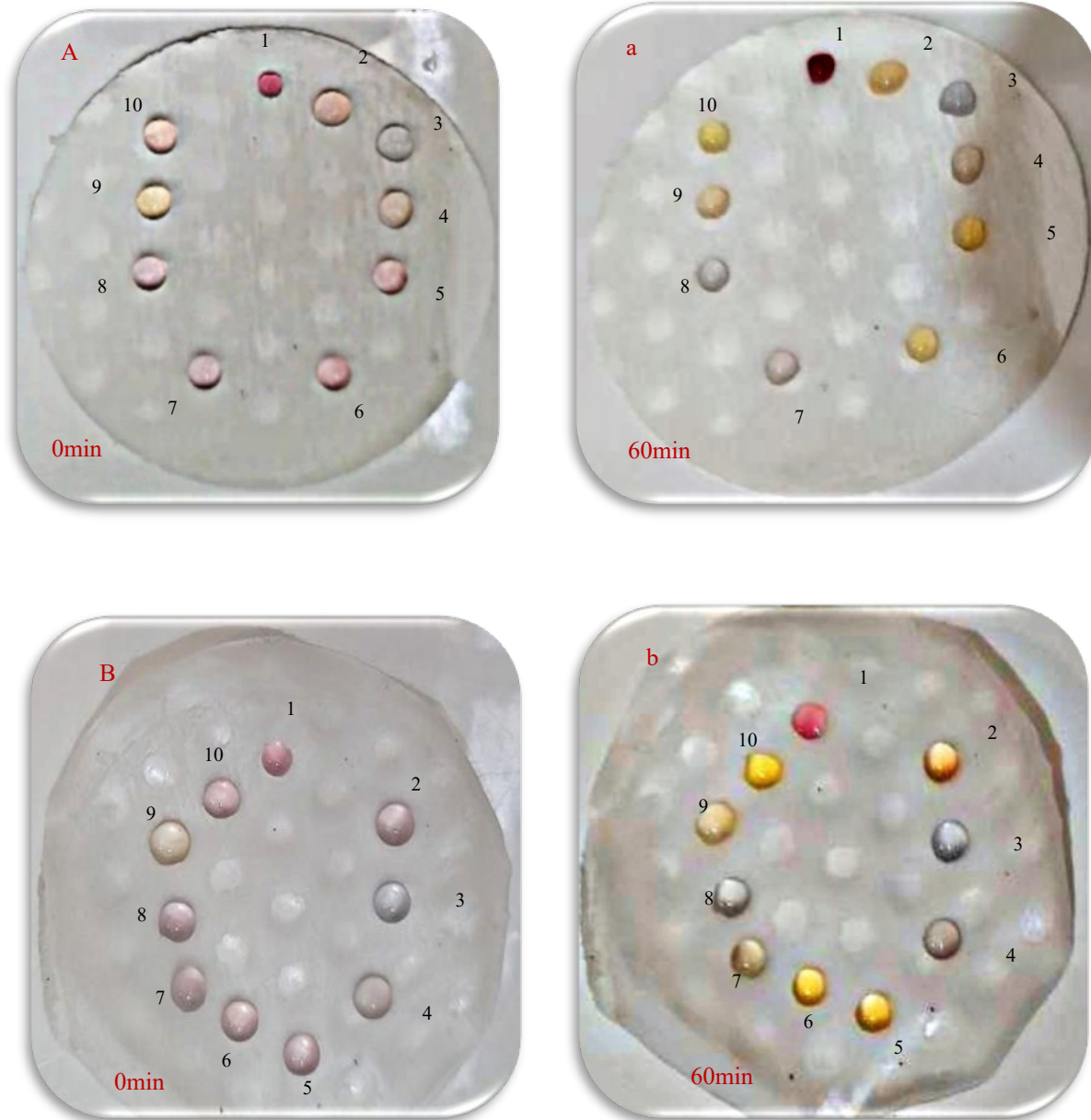
Fig. S6. High-resolution images of \mu PCD and Parafilm for (1) AgNPrs (2) AgNPrs/HA/ Glycine, (3) AgNPrs/ HA /Cysteine, (4) AgNPrs/ HA /Met, (5) AgNPrs/ HA /Pro, (6) AgNPrs/ HA /Phenyl, (7) AgNPrs/ HA /Aspartic acid, (8) AgNPrs/ HA /Ascorbic acid, (9) AgNPrs/ HA /Dopamine, (10) AgNPrs/ HA /urine (1:0.5:0.5 V/V), (A, a). High-resolution images of \mu PCD in 60min, (B, b). High-resolution images of parafilm in various incubation times of 0 and 60min.
