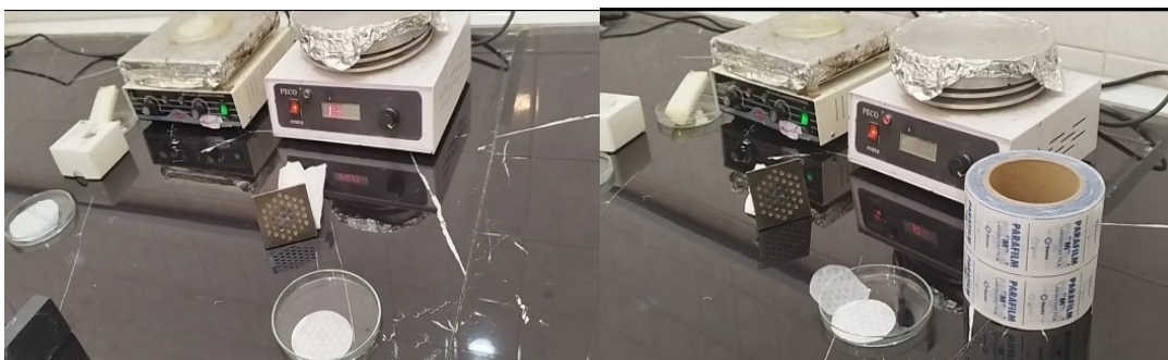
Scheme S1. Photographic images for Paper and parafilm based \mu PAD fabrication.
