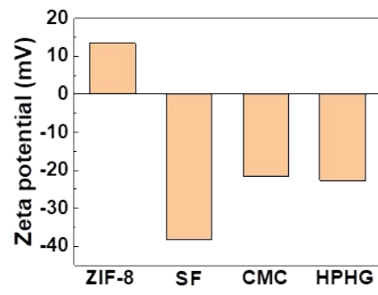
Figure S2. Zeta potential of ZIF-8 aqueous, SF aqueous, CMC aqueous and HPHG precursor.
