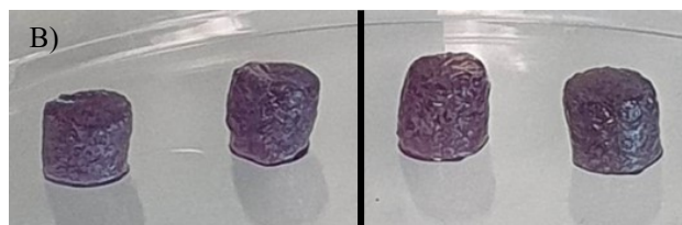
Figure S8. SA 1% CHI 0.75% GNP 0.025% w/v (left) and SA1% CHI0.5% GNP0.025% w/v (right) after (A) 1 week in PBS and (B) 2 weeks in DMEM medium.
