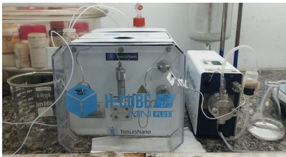
Figure S1. H-Cube® Mini Plus continuous flow hydrogenation reactor (ThalesNano).
