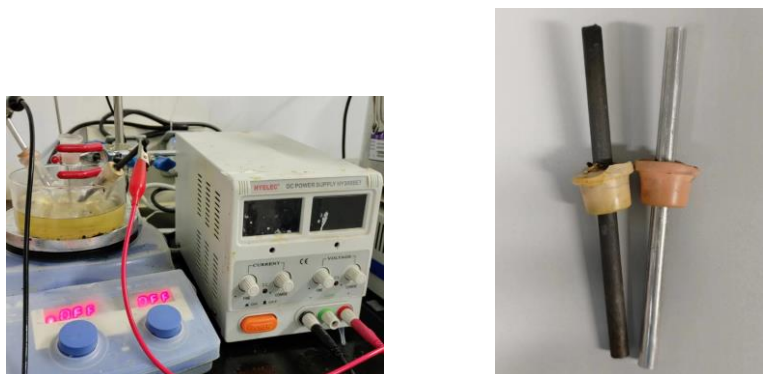
Figure S1 Electrolysis setup
