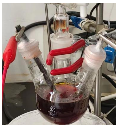
Figure S2 Gram-scale amplification Electrolysis setup
