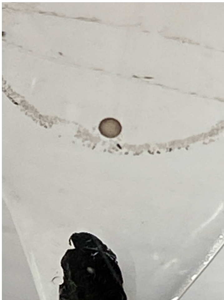
FIGURE S2.1. Sutter's Mill meteorite particle undergoing Folch extraction in a borosilicate glass V-vial. A spherical dark 533 \mu m diameter vesicle of hemoglycin (image lit from the side) has formed at the interphase between the dense chloroform phase and the polar methanol/water phase. The dark object at the bottom of the vial is the particle of Sutter's Mill meteorite from which the polymer diffuses on solvation. The polymer vesicle resides at the interphase because it is less dense than chloroform but denser than methanol/water due to hydrophobic poly-glycine content.
