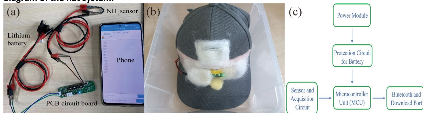
Fig. S9 (a) Wearable NH 3 monitoring system. (b) The practical application of the hat. (c) Circuit diagram of the hat system.
