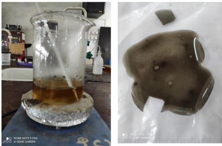
Figure S3: (a) Heating GO / Aloe vera /distilled water mixture up to 80° C (b)Synthesized CMC/GO/Aloe vera composite at 60 °C
