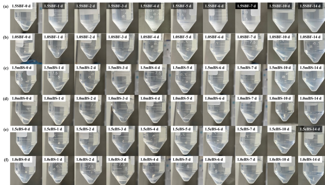
Figure S2 All the appearance on change of the solutions in a polypropylene tube containing slide glass after being kept at 37 °C for various periods up to 14 d.
