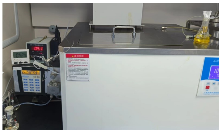
Figure S6. Continuous Packed-bed Reactor III setup (C-H nitrosation of 2-phenylpyridine step)
