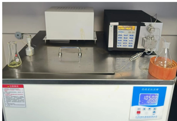
Figure S4. Continuous Packed-bed Reactor I setup (C-H acetoxylation of arenes step)
