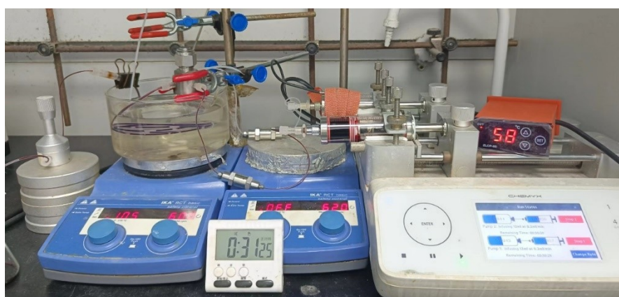
Figure S5. Continuous coil reactor II setup (C-H iodination of 2-phenylpyridine step)
