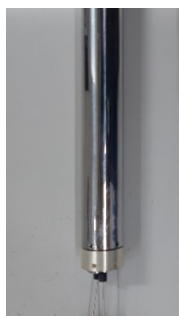
column for HCR-1000, EYELA ID: 37 mm, L: 300 mm
