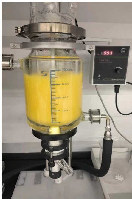
Fig. S1 Digital photograph 840 mL scale oxidation of 2-MN with \text{Ce}^{4+} . The reaction condition: 2-MN (24 mmol) in 240 mL DCE reacted with 600 mL of 0.4 M \text{Ce}^{4+} aqueous solution (containing 3.5 M \text{H}^+ and 4.6 M \text{MeSO}_3^- ) at 65°C, 1000 RPM, for 3h.
