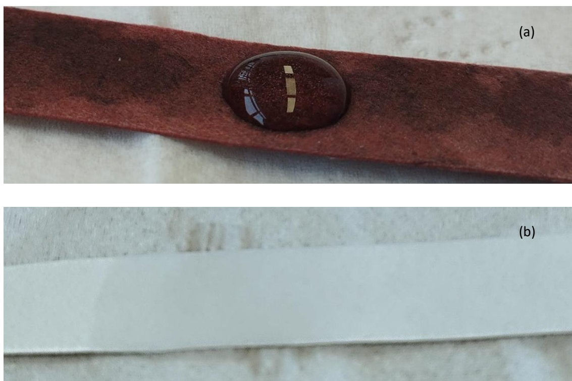
Figure S1. (a) Image of a water droplet deposited on the surface of an AuNW/FP-a strip, showing the water repellency of the surface; (b) Image of a water droplet deposited on the surface of raw filter paper, showing the hydrophilicity of the surface;
