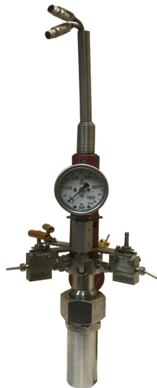
Fig S36. Autoclave for scaling the depolymerization process
