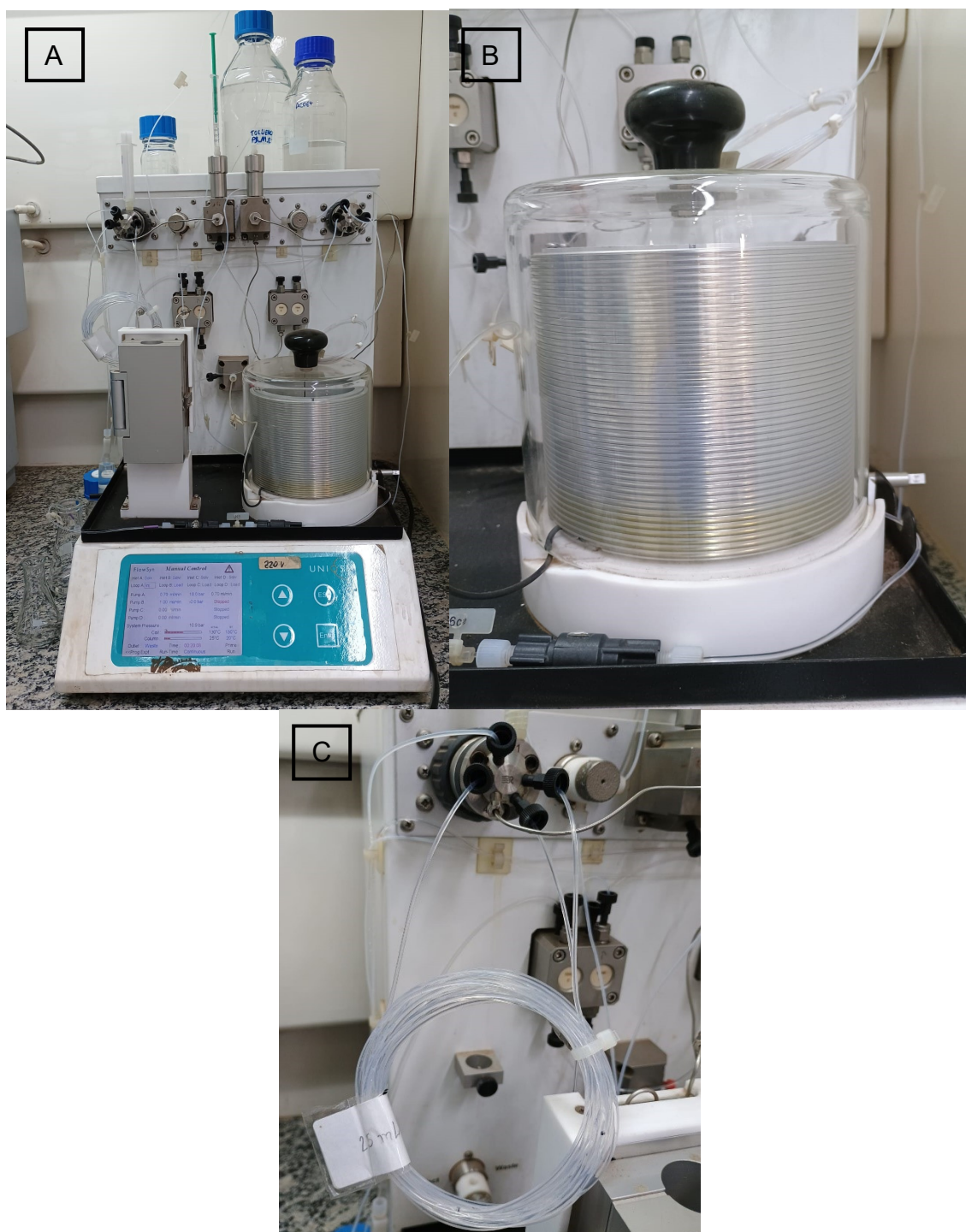
Figure S1. Uniqsis device (a) Picture of full reactor, (b) HPFA Coil reactor (V = 14 mL) and (c) 2.5 mL HPFA coil.
