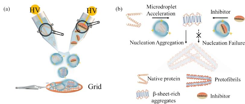
**Fig S11.** Schematic diagrams of (a) the microdroplet reaction system and (b) the mechanism of small molecule inhibitors acting on fibrotic proteins.
