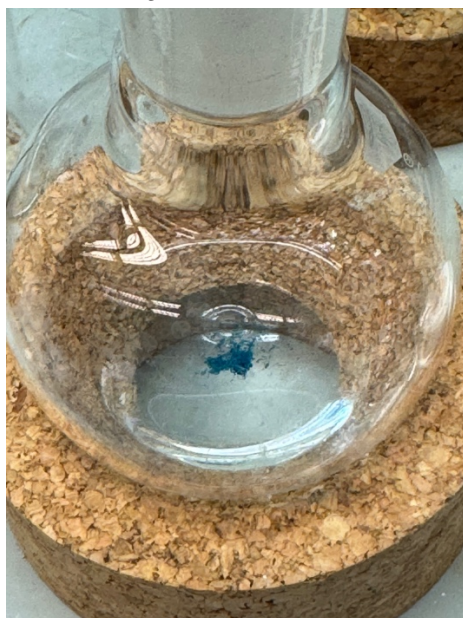
Figure S2: Cu(OAc) 2 in 6 mL (1:5 HFIP:TFT) after sonicating for 10 minutes.
