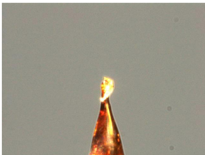
Figure S19: A single crystal of the compound mounted on a loop.
