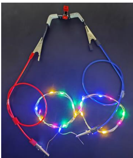
Figure 30. Digital photos of two series P/Fe-HCBA-2-based flexible ZABs powering several LED lights.
